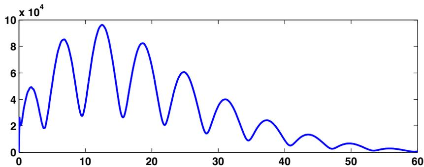
Fig. 5  $\|e^{tA}\|$ , the hump for the stabilized Boeing 767
