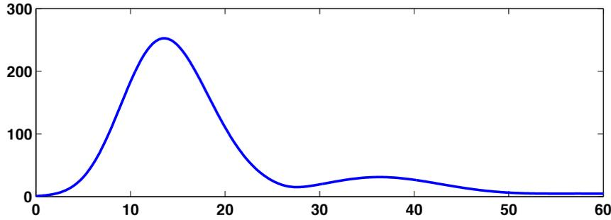
Fig. 3  $\|e^{tA}\|$ , the hump for the transient example
