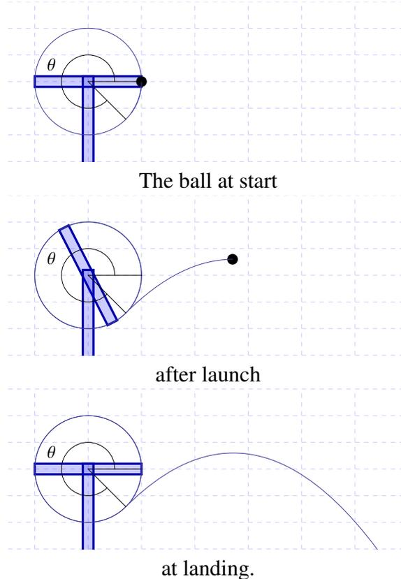
The client has now chosen the values  $r = 11$  cm and  $h = 15$  cm for the final design. Our assignment is to come up with a procedure for specifying  $\theta$  and  $k$  in order to hit a target at a fixed distance  $TD_0 \pm 0.5$  cm from the base of the launcher. We will have to explain to client how to solve for  $\theta$  and  $k$  in order to hit the target, and illustrate our method with some particular examples.
